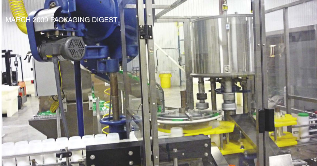
Caps are sorted in a vertical rotary unit and then travel down a chute to a four-station transfer table that transports them to the four-head rotary capper.
