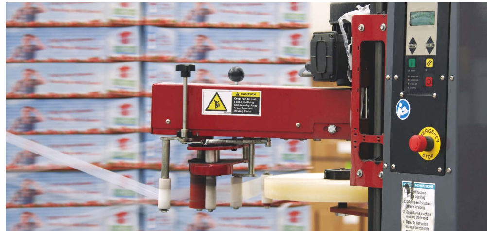
Tape is prestretched to 650 percent before it is wrapped around a pallet of tomatoes.
