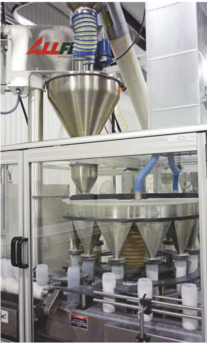
An auger meters detergent into 12 funnels that deliver the product into containers traveling on the rotary turntable.
